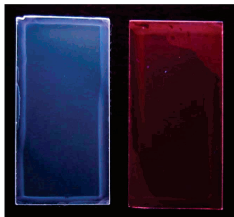
Figure 10. Photographs of oligo( p -phenylene vinylene) amphiphile ( 1a )/poly(2-hydroxyethyl methacrylate) film (left) and 1a /silicate film (right) from precursor solutions containing 2 mol % of rhodamine B derivative ( 2 ) under UV irradiation ( \lambda = 365 nm).
